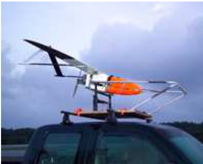
The UAS is launched from a moving platform to rendezvous with an approaching hurricane
